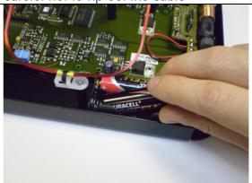
The battery is located in the bottom right hand corner of the base
