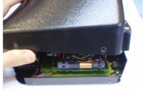
Using the 2mm allen key remove the 4 screws on the side of the UCS
